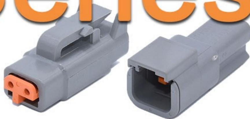
DTM series connectors offer solutions to your smaller wire gauge applications. Building on the DT design strengths, the DTM connector line was developed to fill the need for lower amperage, multi-pin connectors. The DTM series offers the designer the ability to use multiple size 20 contacts, each with 7.5 amp continuous capacity, within a single shell.
