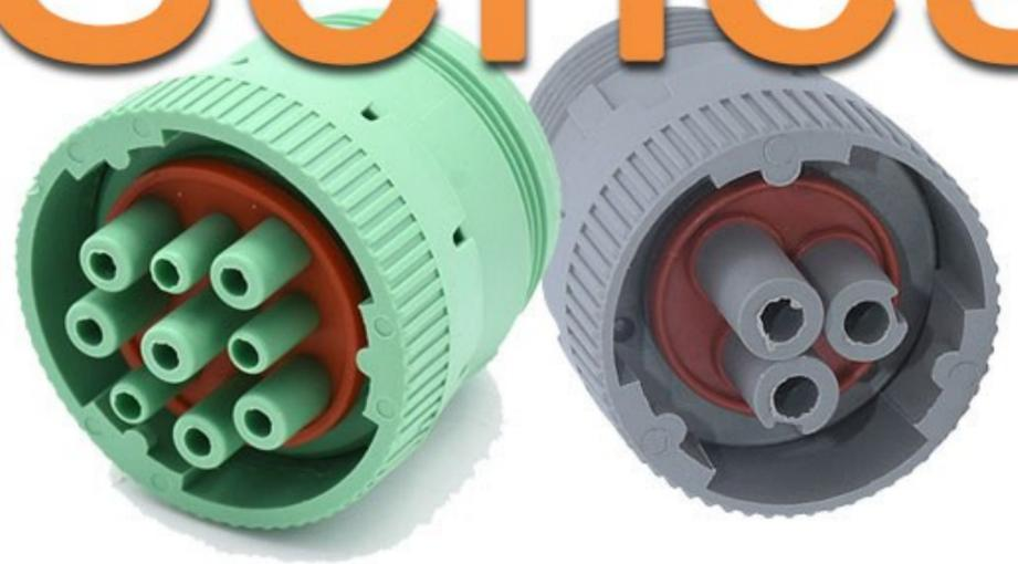
The HD10 series is an environmentally sealed, thermoplastic, and cylindrical connector series. With arrangements from 3 to 9 cavities, HD10 connectors accept size 4, 12, or 16 contacts and are available either in-line or flanged. HD10 connectors are heavily used for diagnostic applications and are available with or without a coupling ring.
